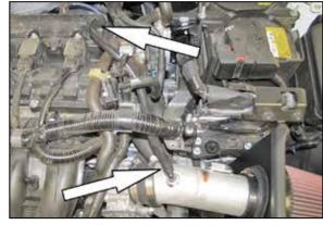
20. Install the provided crank case vent hose onto the valve cover port and then onto the fitting installed into the K&N® intake tube.
