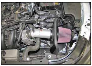
19. Install the K&N® Air filter through the heat shield, install the intake tube into the air filter and then into the coupling hose. Adjust the tube and filter for best fit and then secure with the provided hose clamps.
