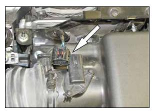
3. Disconnect the mass air sensor electrical connection and unhook the wiring harness from the air box.
