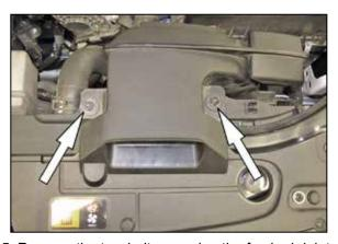
5. Remove the two bolts securing the fresh air inlet duct to the core support.
