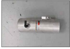
16. Install the provided 90° vent fitting into the K&N® intake tube as shown.
