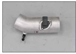
18. Install the mass air sensor into the K&N<sup>®</sup> intake tube and secure with the provided hardware.
