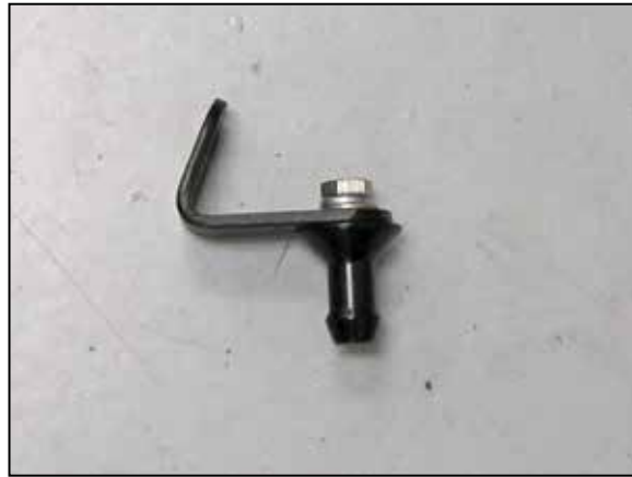
14. Install the mounting stud onto the mounting bracket using the provided hardware.
