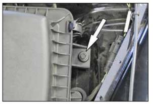
8. Remove the bolt securing the air filter assembly onto the inner fender.
