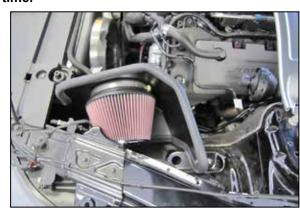
15. Install the K&N® air filter onto the adapter and secure with the provided hose clamp, then secure the heat shield and brackets to the air filter housing mounting location using the provided hardware.
