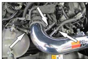
21. Connect the crank case vent, EVAP vent and idle by pass lines to the quick disconnect fittings installed into the K&N® intake tube.
