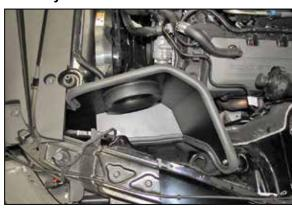
14. Set the heat shield onto the mounting bracket installed in step #9 and secure with the provided hardware.
