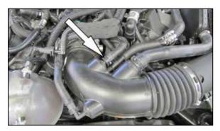
3. Depress the locking tab and then disconnect the idle bypass hose from the intake tube.
