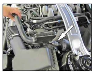
5. Cut the clamp that secures the sound tube/ chamber to the sound drum and then disconnect the sound tube/chamber from the sound drum.
