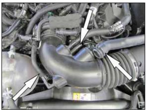
4. Depress the locking tabs and then disconnect the crank case vent hose and the EVAP vent hose. Then release the spring clamp and disconnect the sound tube from the intake tube.
