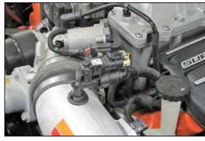
17. Reconnect the crank case vent hose and pressure sensor electrical connection.
