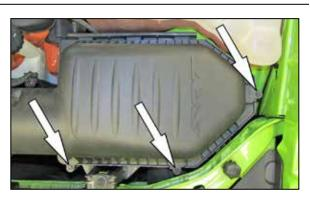
5. Loosen the three screws securing the upper air filter housing and then remove the upper air filter housing and intake tube.
