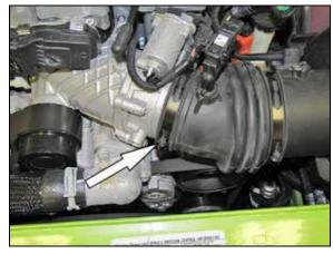
4. Loosen the hose clamp securing the intake tube to the throttle body.
