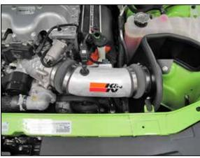
16. Install the K&N® intake tube assembly into position, Slide the coupling hoses out and onto the throttle body and filter adapter. Then adjust the tube and hoses for proper fit and secure with the provided hose clamps.
