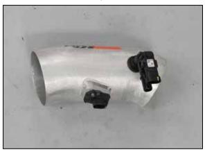
14. Install the provided grommet and pressure sensor/vent assembly into the K&N® intake tube as shown.
