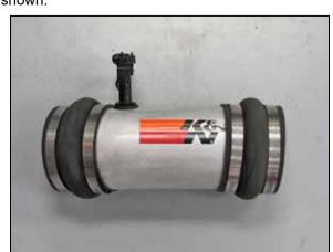
15. Install both of the coupling hoses (08418) onto the  $K\&N^{\circledcirc}$  intake tube as shown.
