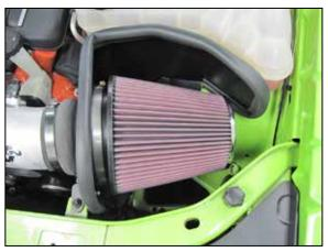
19. Install the K&N® air filter and secure with the provided hose clamp.
