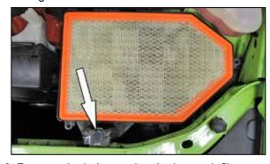
6. Remove the bolt securing the lower air filter housing to the core support and then remove the air filter housing from the vehicle.
