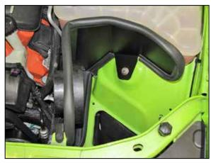
11. Install the heat shield assembly into the vehicle so the insert nut goes into the factory air box grommet mount. Secure the bracket to the core support with the factory bolt from step #6 and tighten the bolt into the insert nut.
