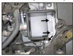
19.Install the heat shield assembly as shown. Secure the heat shield to the air box mounting locations with hardware provided.
