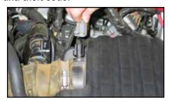
2. Disconnect the inlet air temperature sensor electrical connection.
