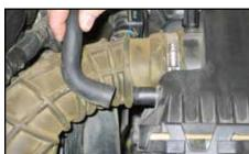
3. Disconnect the crank case vent hose from the upper air box housing.
