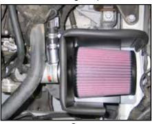
24. Install the K&N<sup>®</sup> air filter onto the intake tube and secure with the provided hardware.
