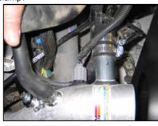
21. Reconnect the inlet air temperature sensor electrical connection.
