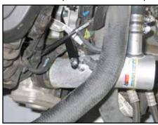
18. Install the K&N<sup>®</sup> intake tube into the silicone hose at the throttle body and align with the bracket installed in step #11. Then secure the intake tube with the hose clamp and hardware provided.
