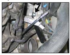
12. On 2010 model year and earlier vehicles, Install the tube mounting bracket (06716) using the provided hardware.
