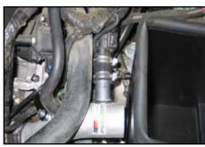
22. On vehicles equipped with an air injection pump, reroute the hose under the engine wiring harness and then connect it to the intake tube and secure with the provided hose clamp.
