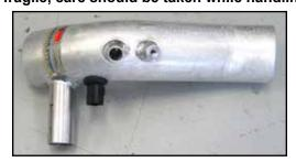
15. Install the air temperature into the grommet installed into the  $K\&N^{@}$  intake tube during step #13.
