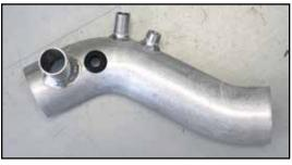
13. Install the provided temperature sensor grommet into the  $K\&N^{\mbox{\scriptsize $B$}}$  intake tube as shown.
