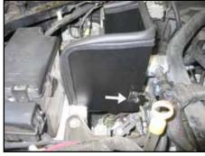
23. Secure the battery cable mounting bracket to the heat shield using the provided hardware.
