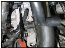
12a. On 2011 and later model vehicles, remove the upper bell housing bolt then install the tube mounting bracket (064307) as shown and secure with the factory upper bell housing bolt.
