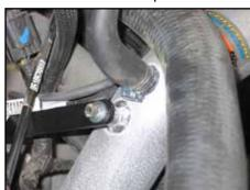
20. Attach the crank case vent hose to the K&N<sup>®</sup> intake tube and secure with the provided hose clamp.
