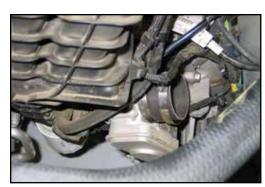
11. Install the provided silicone hose (08284) onto the throttle body and secure with the provided hose clamp.
