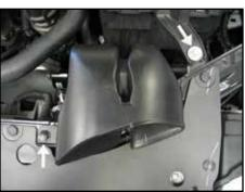
6. Remove the bolt which secures the air box to the radiator core support shown and then remove the plastic retaining clip which secures the fresh air inlet
