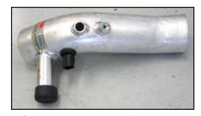
16. On vehicle not equipped with and air injection pump, install the provided vent cap onto the air fitting and secure with the provided hose clamp.
