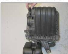
14. Remove inlet air temperature sensor from the stock air box and then remove the o-ring from the sensor.
