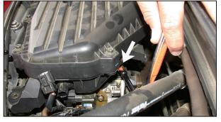
8. Loosen the hose clamp that secures the plenum to the throttle body as shown.
