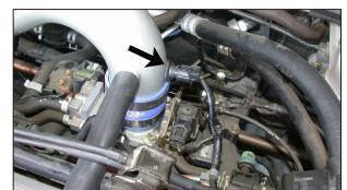
27. Reconnect the air temperature sensor electrical connection as shown.
