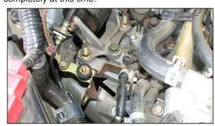
20. Install the remaining rubber mounted stud to the lower resonator mounting point as shown.
