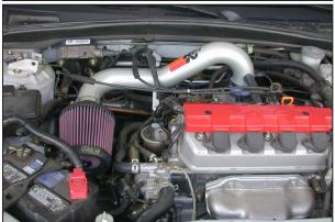
28. This K&N® high flow intake system has been designed to be used in two different configurations. In the case of inclement weather, the cold air tube can be removed and the air filter can be clamped onto the intake tube located in the engine compartment to avoid the possibility of ingesting water into the engine.
