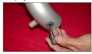
17. Install the provided rubber grommet into the hole on the K&N® intake tube, then install the air temperature sensor into the grommet as shown. NOTE: Before installing the grommet and air temperature sensor, inspect the inside of the tube for any debris, then clean the inside out with water and a towel. Inspect the tube one more time before proceeding to the next step. NOTE: Take care when handling the temp sensor as it is very fragile.
