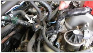
15. Install the rubber mounted stud onto the stock resonator mounting location as shown.
