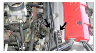
13. Secure the throttle cable and cruise control cable (if equipped) to the stock clips as shown.
