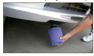
25. Raise the vehicle up and support it with jack stands, then, install the K&N<sup>®</sup> air filter from underneath the vehicle as shown.
