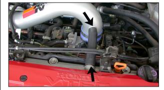
26. Install the provided silicone hose onto the crank case vent on the cam cover, then connect the other end to the vent on the K&N® intake tube as shown.
