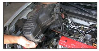
12. Unclip the throttle cable and cruise control cable (If equipped), then, remove the resonator by pulling upwards as shown.
