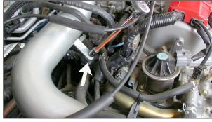
19. Secure the bracket to the rubber mounted stud using the provided hardware, but do not tighten completely at this time.
