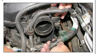
11. Using a flat blade screwdriver, unclip the wire harness from the resonator as shown.
