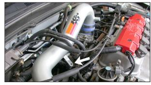
18. Install the K&N® intake tube onto the throttle body, then, line up the bracket with the rubber mounted stud as shown. Tighten hose clamps at this time.
