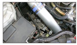
23. Slide the K&N® cold air tube onto the throttle body tube and line up the bracket with the rubber mounted stud as shown and secure with the provided hardware. Do not tighten completely.
