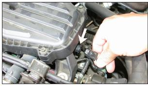
2. Disconnect the air temperature sensor electrical connection as shown.
