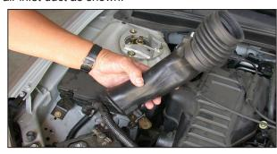
5. Remove the air inlet duct.
