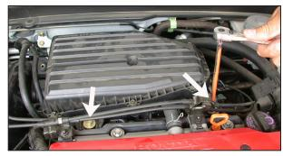
7. Loosen and remove the two bolts that secure the throttle body plenum.
