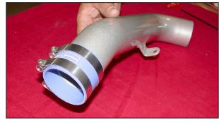
21. Install the silicone hose and hose clamps onto the K&N® cold air tube as shown.
