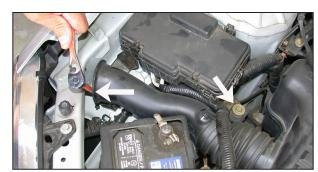
4. Loosen and remove the two bolts that secure the air inlet duct as shown.
