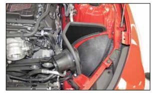
11. Install the heat shield so that the mounts snap into the factory air filter housing mounts.
