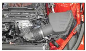
4. Loosen the hose clamp at the throttle body and then remove the complete stock intake system. NOTE: The air filter housing is snapped into three grommets.
