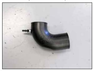
14. Install the provided NPT quick disconnect fitting into the K&N® intake tube as shown.
