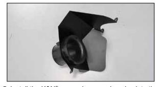
5. Install the K&N $^{\!0}$  mass air sensor housing into the Heat shield and secure with the provided hardware.
