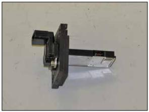
22. Install the mass air sensor into the provided adapter and secure with the provided hardware.
