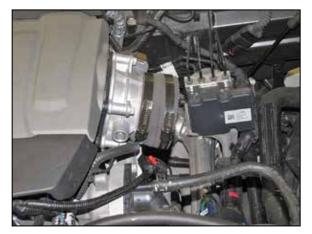
19. Install the provided coupling hose (08761) onto the throttle body and secure with the provided hose clamp.
