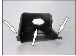
16. Install the 16" section into the hole of the heat shield and install the 27" section around the perimeter of the heat shield as shown.
