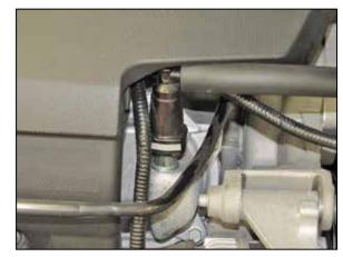
4b. On vehicles equipped with a "Wet Sump" oiling system, disconnect the crank case vent hose from the passenger side valve cover port and remove the hose from the vehicle.
