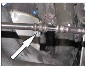
12. Using a razor knife, cut the plastic hose at the TEE fitting where shown. Separate the plastic hose from the TEE fitting.
