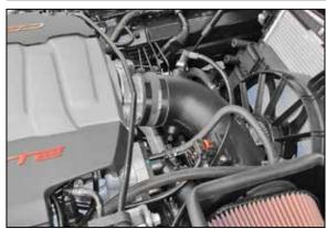
26. Connect the crank case vent hose to the fitting installed into the K&N $^{\odot}$  intake tube as shown. NOTE: On vehicles that are not equipped with
