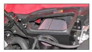
18. Install the heat shield assembly onto the rubber mounted studs and secure with the provided hardware.
