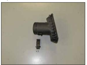
20. Remove the two screws securing the mass air sensor to the factory housing and then remove the sensor from the housing.
