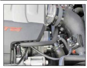
31. Reinstall the 90° quick disconnect fitting onto the valve cover port and then connect the open end of the hose to the fitting installed into the K&N® intake tube.
