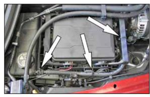
13. Install the provided coolant hose assembled from step #10 onto the expansion tank. Route the coolant hose and then attach the open end onto the TEE fitting and secure with the provided spring clamp. Use the provided tie wraps to secure the coolant hose.
