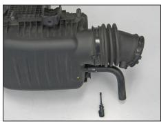
15. Remove the inlet air temperature sensor from the factory intake tube as shown.
