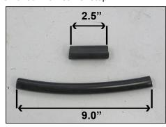
19. Cut the provided ½" silicone vent hose to a length of 9" long, and cut the 5/8" vent line to a length of 2.5" long.
