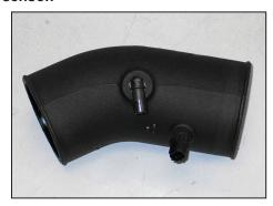
17. Install the provided 90° vent fitting into the K&N® intake tube as shown.
