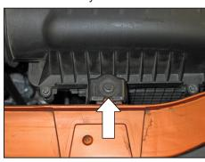
6. Remove the bolt that secures the air box to the core support.
