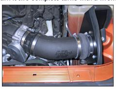
18. Install the K&N® intake tube into the silicone hump hose and then into the silicone step hose at the throttle body. Align the intake tube and heat shield for proper fit and then secure the intake tube with the provided hose clamps and the heat shield bracket with the factory air box retaining bolt removed in an earlier step.
