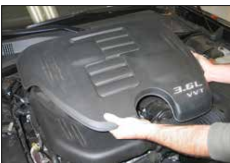
2. Lift up and remove the engine cover.
