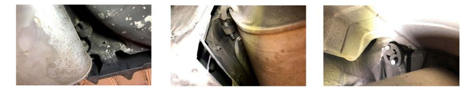
4. REMOVE THE MUFFLERS FROM THE VEHICLE (BOTH SIDES)
