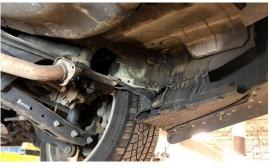
4. REMOVE 2 BOLTS SECURING YOUR STOCK Y PIPE TO YOUR DOWNPIPE
