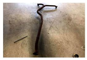
6. INSTALL NEW MAP MIDPIPE, SECURING IT WILL INCLUDED HARDWARE AND GASKETS, REINSTALL RUBBER HANGERS
