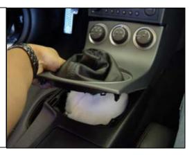
3. Unplug wiring harness from console plate and remove console plate.
