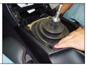
23. Reinstall white foam (350Z and G35 only) and console plate, making sure to re-plug in wiring harness.
