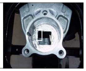
13. If you were unable to remove the shift knob in step 1, then carefully place the knob in a vise (shifter inverted) and using the long extension or other long tool through the lower connection hole, carefully rotate (unscrew) the shifter assembly off of the shift knob.
