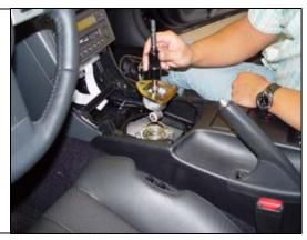
12. File out approx.125" from shifter casting in indicated area. Clean out metal chips and relube entire pocket with provided grease.
