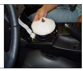
5. Remove shifter cover bolts and wire harness connections, then remove plate from vehicle.
