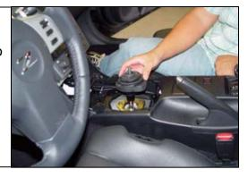
7. Remove bolts holding down metal shifter plate.
