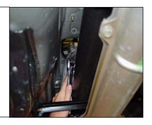
11. Remove shifter from car. (Metal plate and spring will be used on new shifter)
