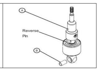
15. Install mounting plate **E** on shifter, make sure that reverse pin is lined up with cleared out area on plate as shown.
