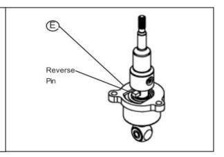
16. Install stock spring and shifter using stock plate and M6 bolts, washers, then serrated washers D. Make sure that reverse pin is turned towards passenger side of vehicle. TOOLS: Socket Drive, Extension, and Hex Drive (5 mm)
