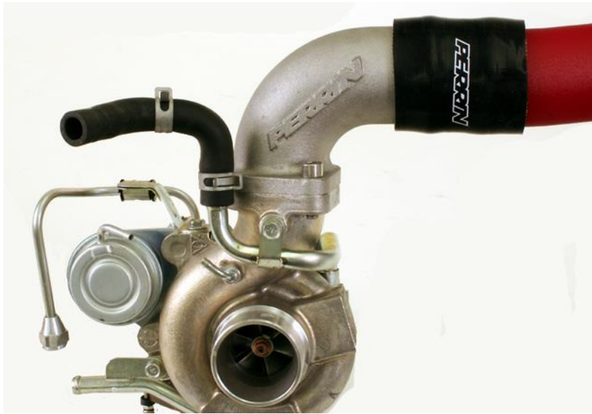
Pic shows adapter bolted to turbo, make sure to use silicone gasket sealer between flanges
