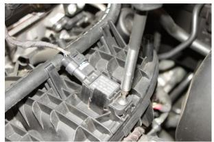
2. Remove sensor mounting screw using T20 torx, then push outward on retaining taps and pull out sensor from intake manifold.
