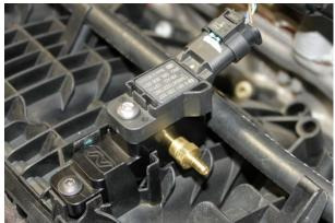
5. Lightly oil "O" ring on original boost sensor and install into *NEUSPEED* Boost Tap, tighten using supplied M6x14mm SS button head screw.
