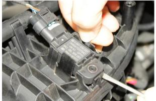
3. Push side retaining clips outward, and then pull out boost sensor from intake manifold.
