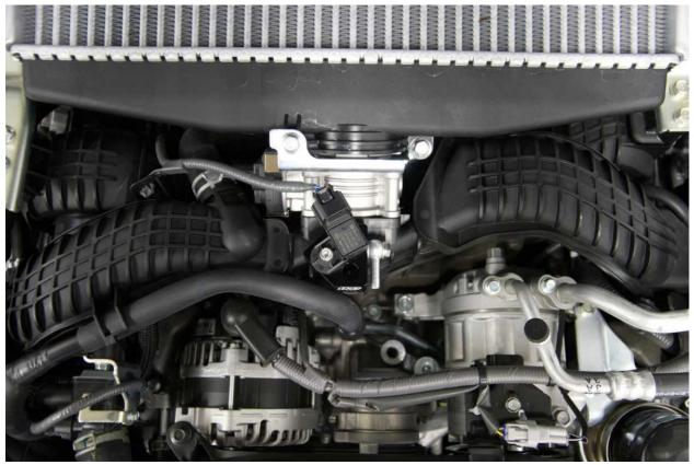
See the routing of the hose through here, then pass the hose down to the turbocharger area. We chose to run the line under the pcv hose pictured below.
