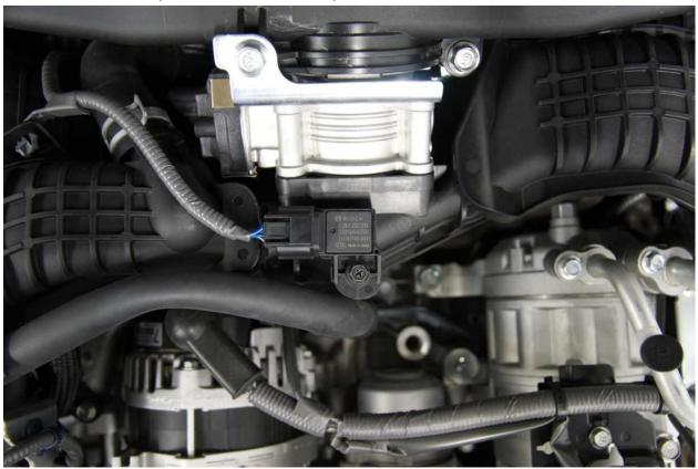
Install the Vacuum Adapter. You will re-use the phillips head screw to attach the adapter. Then attach the MAP sensor to the adapter.
