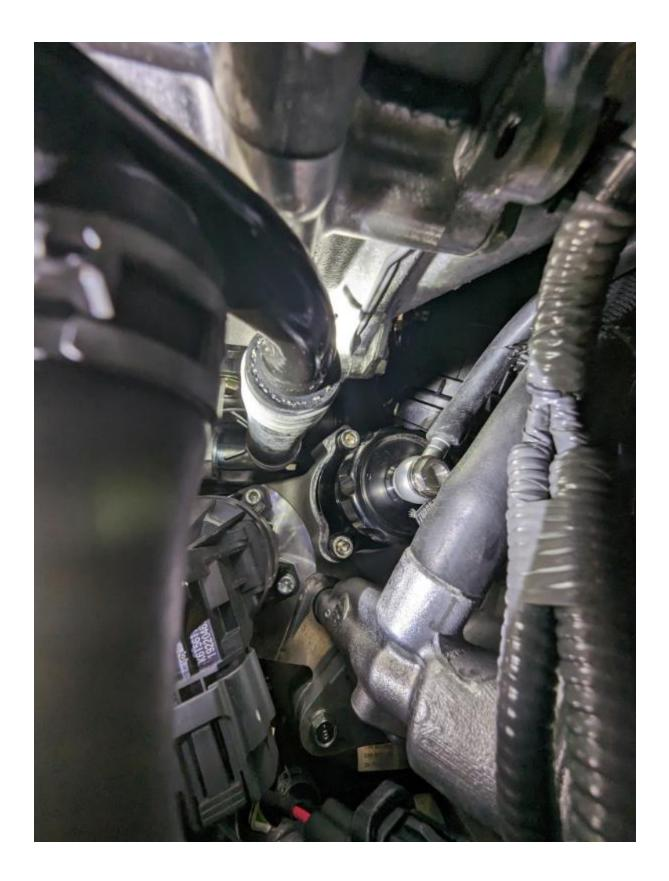
Run the vacuum line to the top of the valve. Make sure to route hose away from moving parts. Do not forget to make sure the 10mm hose barb at the top of the valve is tight and the cap is tight (remember this is not an adjustment). Check your install and secure the hoses with the zip ties supplied.
