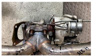
13. INSTALL TURBO ONTO THE MAP HEADER, REUSING THE NUTS YOU REMOVED OFF FACTORY MANIFOLD, YOU NEED TO USE A COMBINATION WRENCH TO TIGHTEN THESE NUTS
