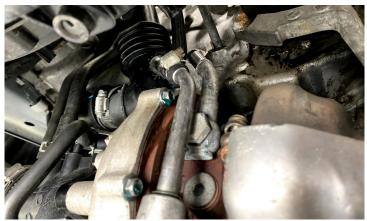
11. REMOVE ENTIRE TURBO AND MANIFOLD ASSEMBLY FROM ENGINE BY REMOVING 6 14MM NUTS FROM THE STUDS HOLDING IT IN PLACE
