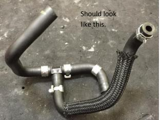
5. Replace the OEM vacuum line going from the 'T' to the wastegate with a piece of 6mm (1/4") vacuum line. This piece of stock vacuum line contains a secondary restrictor pill that results in underboosting when a vehicle is upgraded with exhaust modifications and running a Stage 1+TBE or greater map. You could also remove the pill from the OEM vacuum line if you choose.
