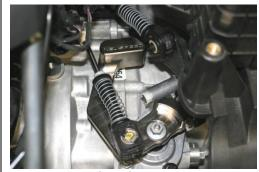
Grease guide rail on NEUSPEED® gear selector lever. Install selector lever by first installing guide rail in white plastic guide. Then match up splines on selector shaft – note wide alignment spline. Install lock nut and torque to 20 ft./lbs. Grease pin on gear selector lever and re-attach cable and retaining clip.
