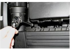
Using a 5mm hex key wrench, unbolt air filter box mount, located on back side.
