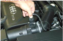
Disconnect Mass Air Flow (MAF) sensor electrical connector.
