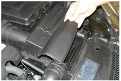
4. Remove cover at intake duct.
