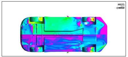
Figure 1.3.2: Cp Plot (Top) of the Diffuser and Splitter
