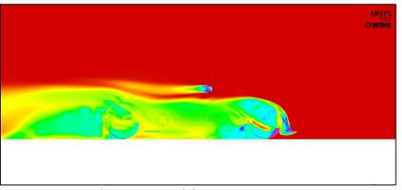
Figure 1.3.8: CpT Plot at Front Endplate
