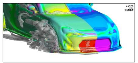
Figure 1.3.5: Q-Criterion Close Up on Front
