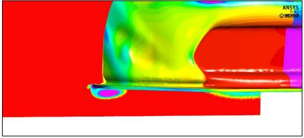
Figure 1.3.7: CpT Plot Just Forward of Front Endplate
