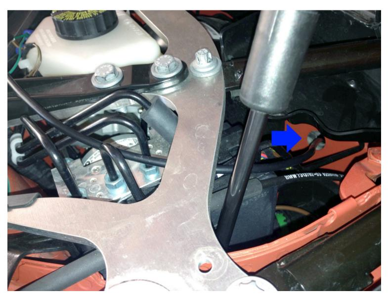
Note if equipped with a manual transmission the clutch line is routed through the same grommet. You can push it out of the way to route the wire or use a wire hanger or similar to push it through.
