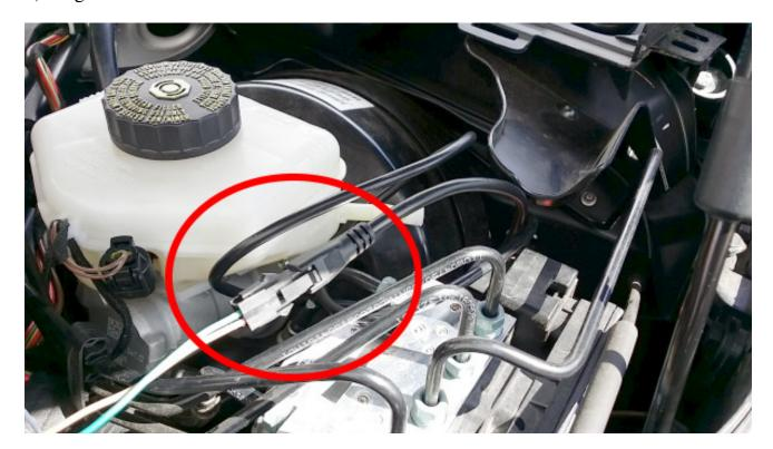
7) Reinstall the interior panel and route the OBDII connection to the OBDII plug with the wire tucked behind the panel you've reinstalled.
