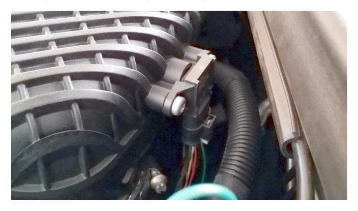
The second connection for Stage1 is the MAP connection. This one is more difficult to reach and will take some patience. If you have larger hands you may also need to temporarily unscrew and push the intercooler water reservoir out of the way to make additional space to reach the sensor. Like the TMAP sensor unplug the OEM connector, plug the JB4 brown patch in to the sensor, and plug the OEM connector in to the JB4 harness.
