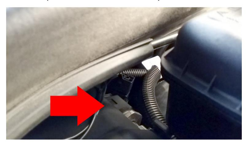
The last connections are to the electronic wastegates. Note that these connections are only utilized for maps 6+ when running more than 25psi and we don't suggest installing them if you only plan to run lower maps.
