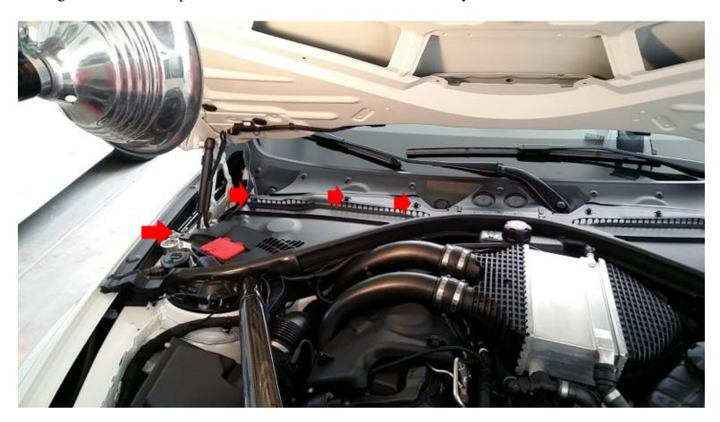
The JB4 control box will sit under the aluminum brace. We suggest using a zip tie to hold it up. Route the harness under the rubber grommet as shown. Note we've covered the jumper battery post with a
