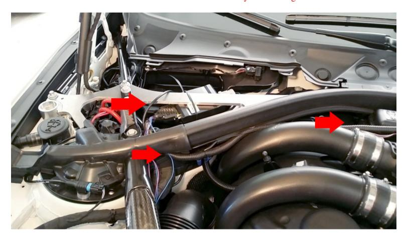
The first connection for Stage1 is to the TMAP connection. Unplug the OEM sensor, plug the JB4 rainbow patch in to the sensor, and plug the OEM plug in to the JB4 harness.
