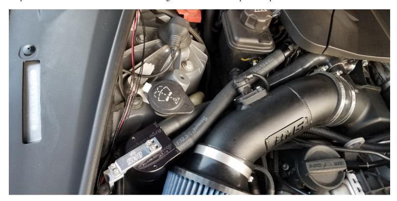
On the other side the hoses won't cross. The straight hose with the billet adapter goes in the "IN" nipple of the catch can and straight into the PCV hose as shown blow. The curved hose connects to the intake. Check all connections and bolts.
