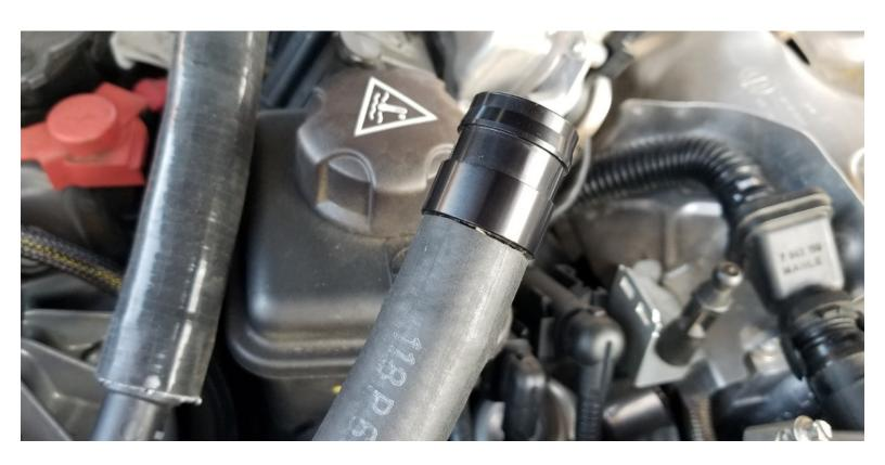
Curved silicon hose goes over PCV nipple on the intake inlet.
