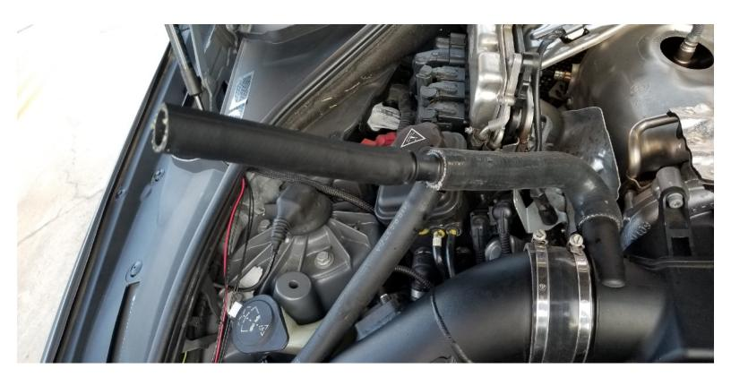
The straight hose with the billet adapter clips into the factory PCV hose. These hoses must cross each other as show in the photo below. Curved hose on the bottom. Straight hose with billet adapter on top.
