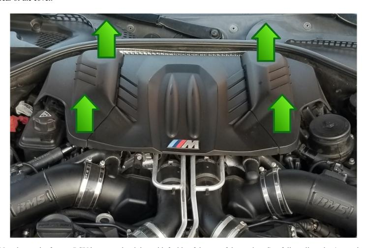
Now locate the factory PCV hoses on the right and left side of the top of the engine. Carefully pull on the 4 pry tabs and pull the PCV hose off.
