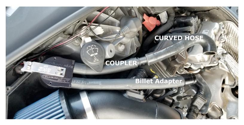
The BMS bracket bolts to the factory intake lower airbox mount next the the fender. Remove the airbox screw, put the BMS bracket in and replace the screw. Bolt in the can and adjust as necessary.
