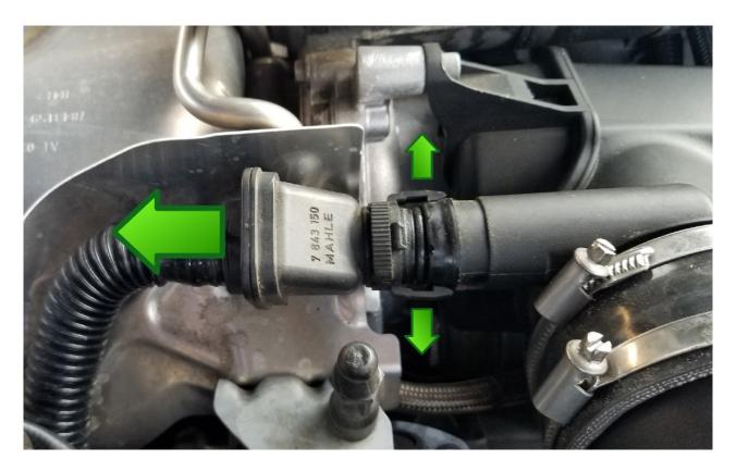
Starting from the left side (looking at the engine) attach the hoses, couplers and billet adapter.
