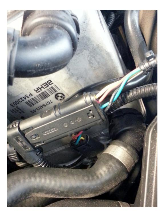
5) Repeat this process for the passenger side TMAP sensor. Note on the passenger side there is a little less room to work with so expect to get a bit frustrated the first time as you release the OEM plug from the sensor and then connect it to the Stage1 harness. Don't worry, it fits, and once you've done it once it will be much easier the second time.
