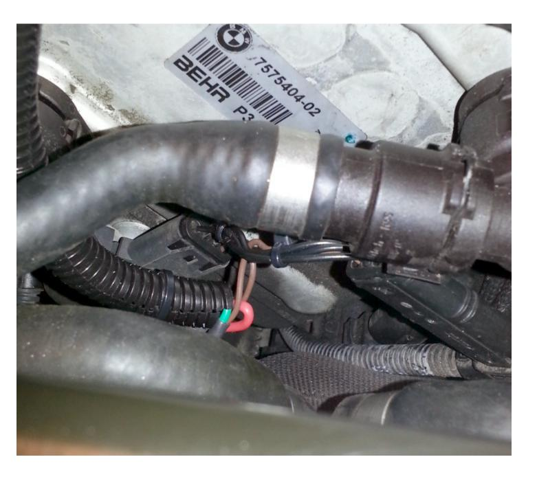
6) Tuck the Stage1 harness out of the way under the rail as shown.
