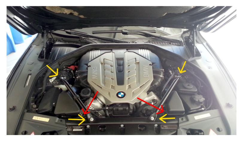
1) Remove the strut brace retaining bolts indicated by the yellow arrows above. With the bolts removed the strut braces lift out of place and will allow easier access to TMAP sensors mounted to the intercooler cores.
