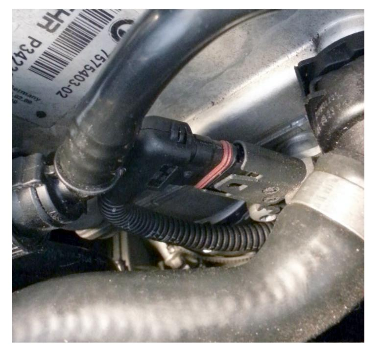
4) Once unplugged push the Stage1 harness male connector in to the TMAP sensor and plug the original male plug in to the Stage1 harness female connector as shown. The rainbow patch will connect to the passenger side sensor while the longer brown patch will connect to the driver side sensor. This allows a passenger side control box placement. Note these photos reflect a driver side control box placement which is no longer suggested.
