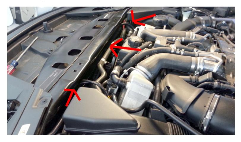
The control box will be placed under the passenger side cowl cover. Connect the Stage1 control box to the Stage1 harness. Lift up the rubber seal and pull back the rubber grommet to route the wire bundle in to the covered area as shown. After the box has been placed push the plastic cowl cover back down over the box. The box fits snuggly and will not rattle or move around. It's normal for the cover to bulge up slightly with the control box below it.
