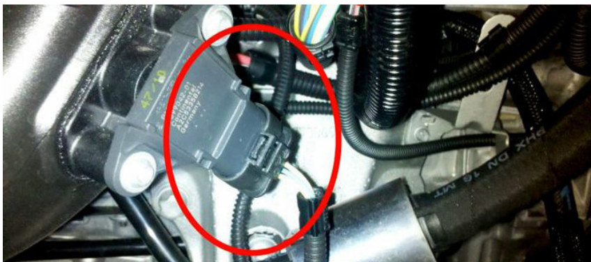
TMAP SENSOR LOCATED ON THE RIGHT SIDE OF THE ENGINE BETWEEN THE AIR BOX AND STRUT TOWER
