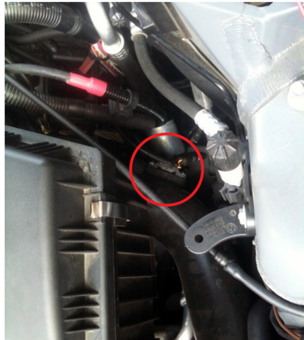
TMAP SENSOR LOCATED ON THE RIGHT SIDE OF THE ENGINE BETWEEN THE AIR BOX AND STRUT TOWER
