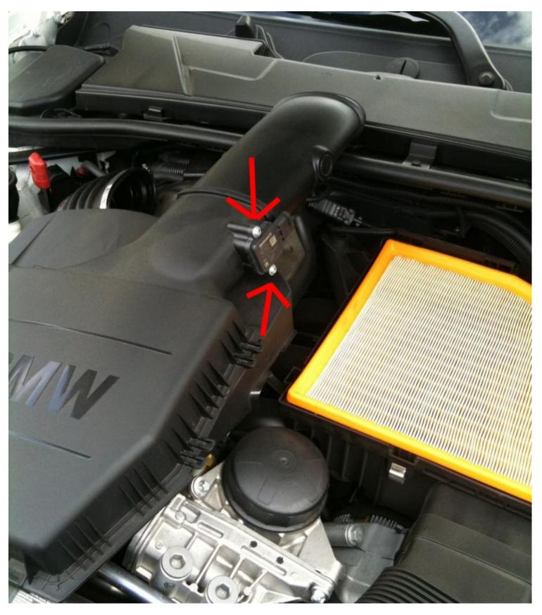
Step 2: The MAF sensor will be removed from the OEM intake and reinstalled in the BMS intake. Remove the two T25 torx screws holding the sensor to the intake tube and pull it straight out.
