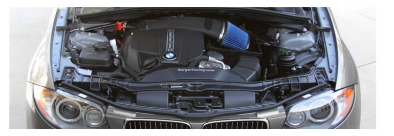
Before you begin open the hood, lock the doors, and wait 10 minutes for the DME to go to sleep. If you have comfort access place the keys at least 30' away from the car. This will avoid triggering a MAF sensor code when the sensor is unplugged during the install process.
