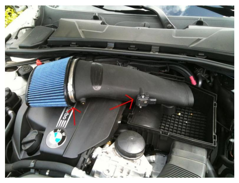
Step 4: Remove the OEM air filter. Remove the 4 silver metal clips from the OEM airbox bottom by bending them down, and then folding them back up, and sliding them down. Keep these in a safe place for when you reinstall the OEM intake. This might also be a good time to vacuum any debris out of your airbox bottom!
