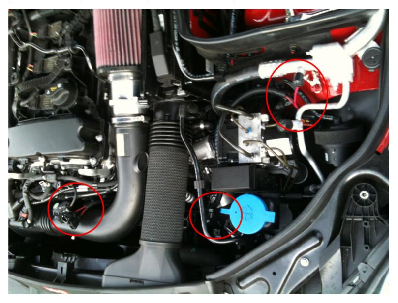
3) Locate the MAP sensor and remove it's plug by pulling the gray clip out approx 1/8" and then pushing it in while pulling the connector out.
