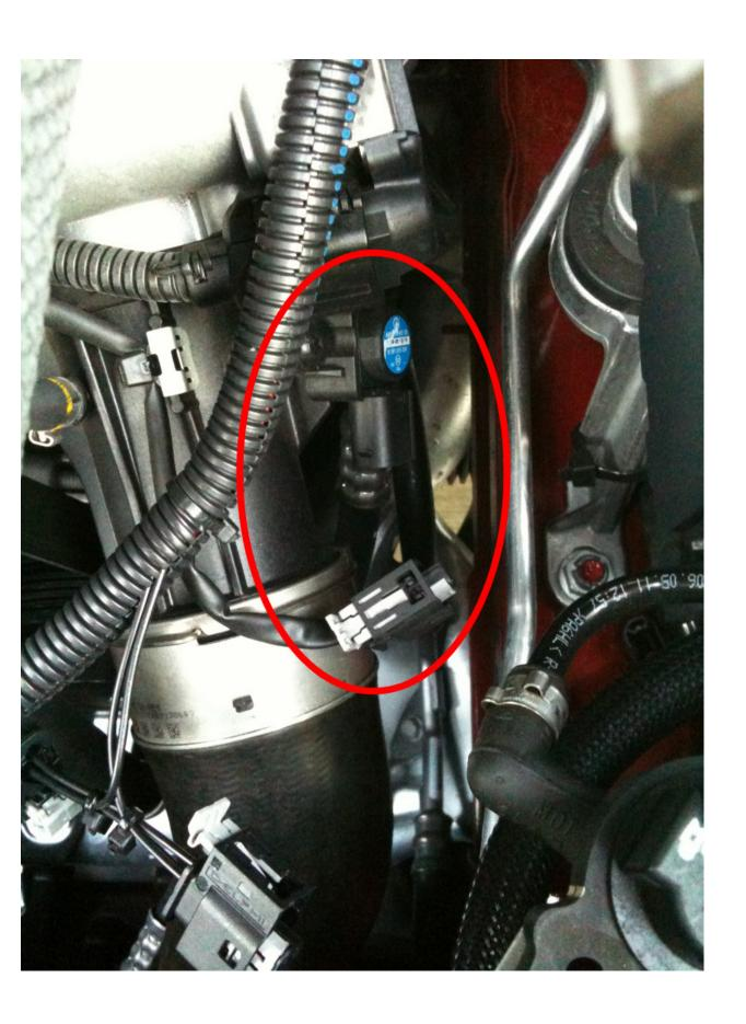
4) Insert the matching JB+ female connector in to the original sensor. Then plug the original connector in to the JB+ connector with 3 male pins sticking out of it. This connector is a simple friction fit and does not require anything to stay
