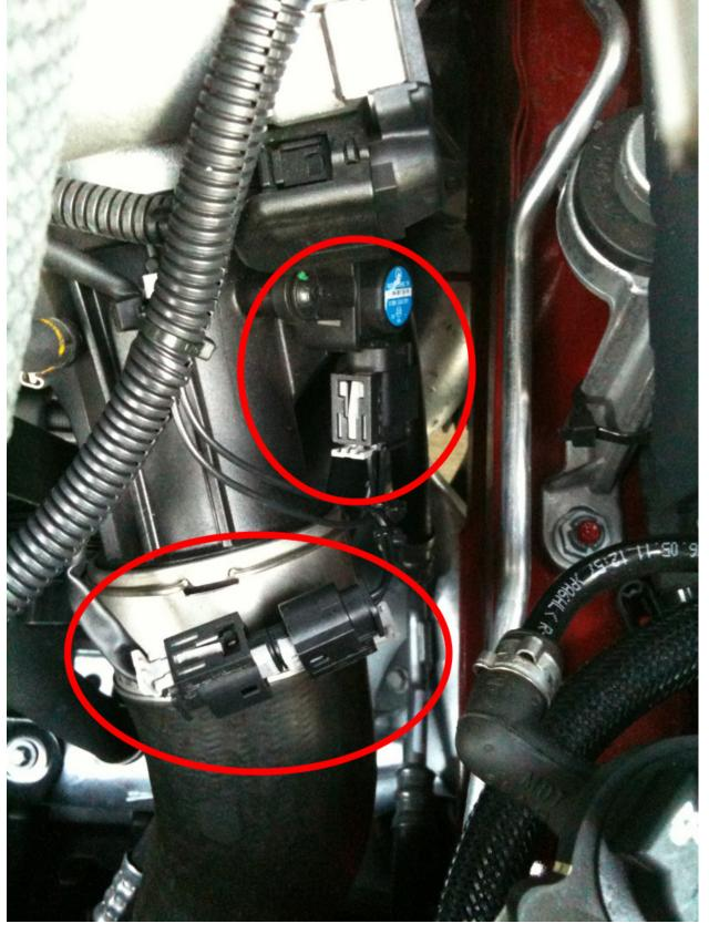
5) Locate the solenoid at the center front of the engine and remove it's plug by pushing in on the metal clip sides while pulling it out.
