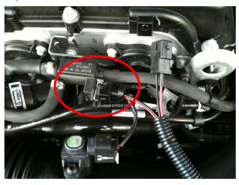
7) Plug the JB+ male connector in to the original solenoid connector.
