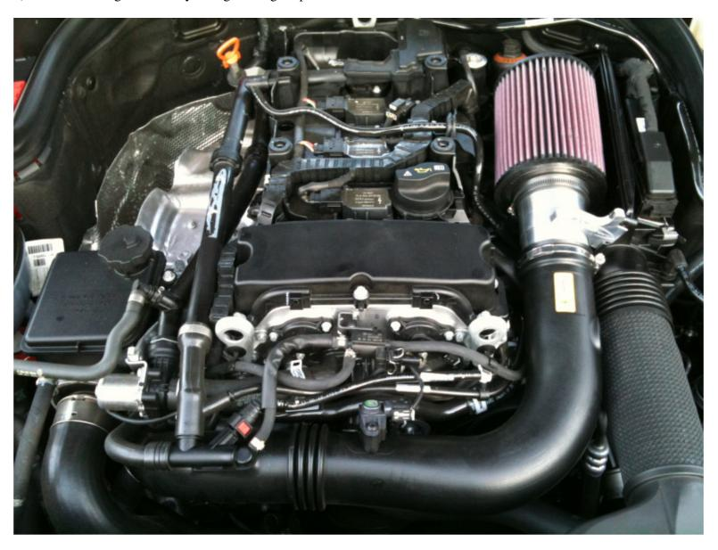
2) Position the JB+ in the install location as shown and route the harness loosely. Using a 10mm socket loosen the ground nut, red in this photo, slide the JB+ ground under the nut, and tighten it.
