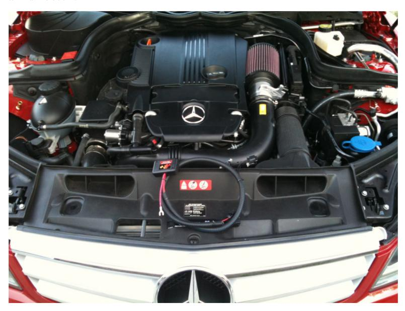
1) Remove the engine cover by lifting it straight up and off.
