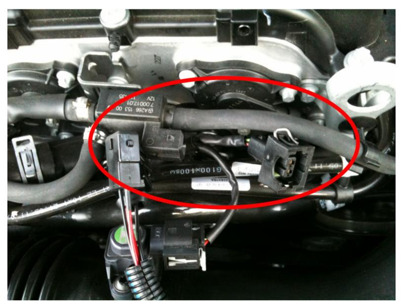
6) Plug the JB+ female solenoid connector in to the solenoid.
