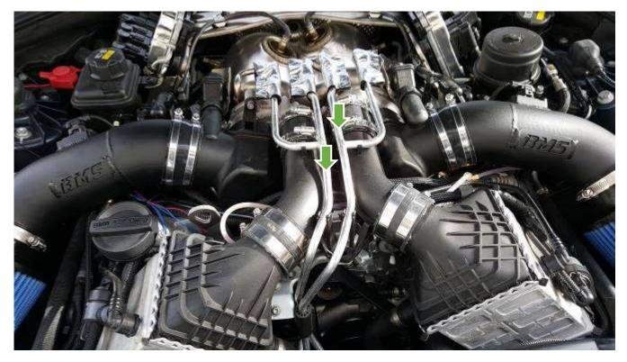
Engine cover removed. Just pull it up. Unscrew the clamps from chargepipe
