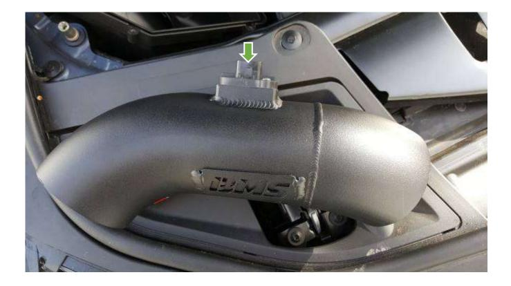
Install the coupler on the turbo side and tighten the clamp.
