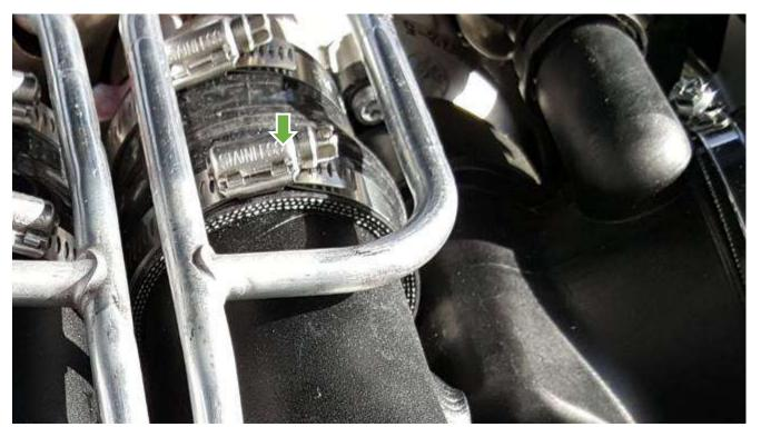
Push the coupler back into the chargepipe and pass the bead roll  $\frac{1}{2}$  an inch or more if possible.
