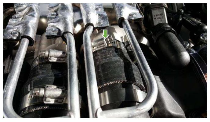
Pull the chargepipe closer to the intercooler as much as possible.
