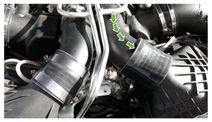
Tighten the second clamp from turbo side.
