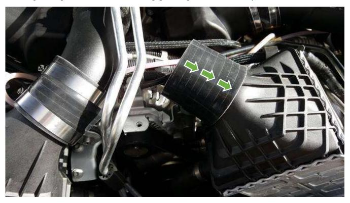
At this step both OEM chargepipe are still off the car and BMS is not installed. Fit the right side (driver side) chargepipe first.
