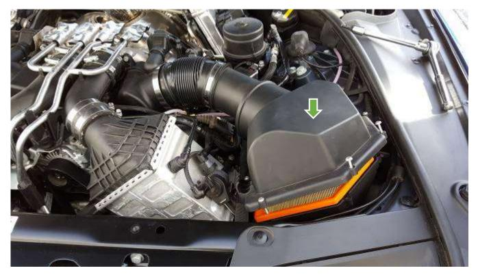
Remove snorkel. Leave the intake under tray intact.
