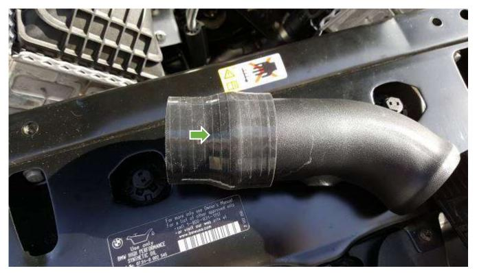
Insert straight coupler into the intercooler pipe and push it all the way in.
