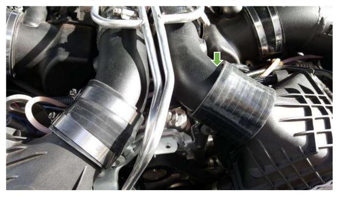
Tighten the clamp on the turbo side. Make sure it's fully inserted.
