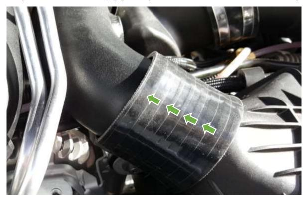
Tighten the clamps on chargepipe and intercooler. Notice how clamp is seated flush on the pipe passed the bead roll.
