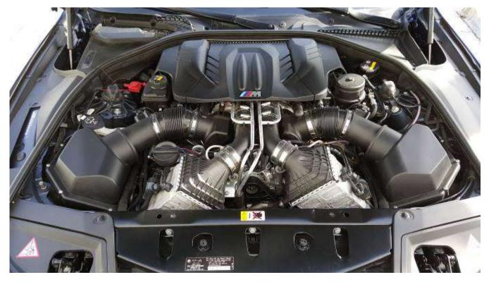
Unscrew the bolts from the intake as well as the clamp on the left.
