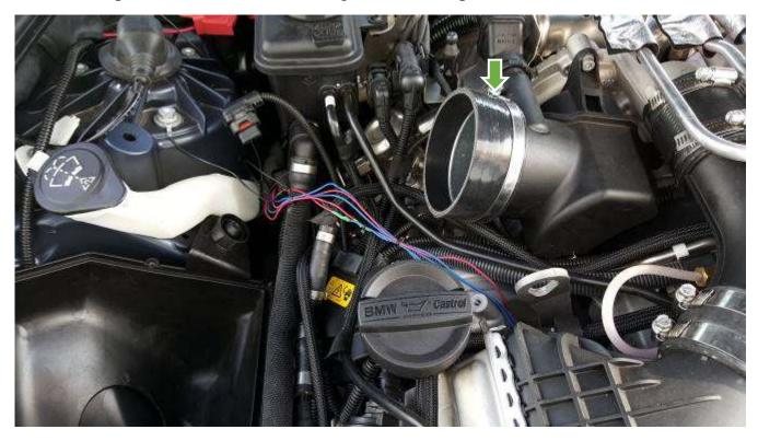
Install the filter on to the pipe. Don't tighten the clamp.
