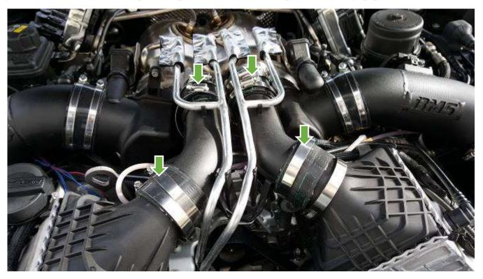
Remove lines from the holding brackets.
