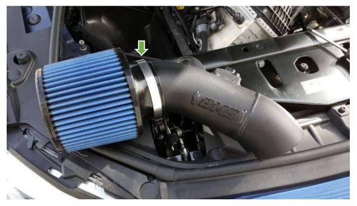
Install intake. Position it similar to the photo below with logo facing towards the front of the car. Tighten the clamp on the turbo side first, then position the filter and tighten the clamp on the filter. Connect MAF sensor. Filter should be 75% in the under tray.
