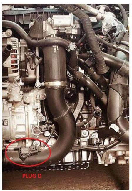
Plug D is found on the charge pipe which goes to the throttle body. It is visible by looking down past the throttle body and is the plug with the brown, yellow , red and grey wires and is the lower plug of the two in the area. (There is a plug with a visible yellow wire in the same location which connects to the air-con pump with two large silver pipes exiting coming up from this).
