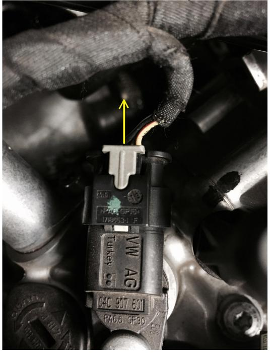
PLUG B: The boost sensor plug on the manifold is removed by pushing the grooved tab down on the end of the sensor (yellow square) and pulling the plug towards the back of the car. Plug the removed plug into the male plug on the JB harness and the female plug from the JB harness into the sensor.
