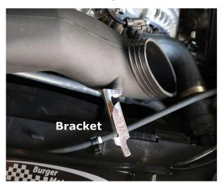
3. Remove the MAF sensor by unscrewing the 2 T20 Torx screws. Remove the vacuum hose to the left of the MAF sensor by squeezing the outer ring and pulling it off. Then carefully pull directly up on the intake. Once off remove the rubber bushing and transfer it to the BMS Performance Intake.
