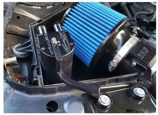
Attach the oil catch can and bracket as shown in the photo to the left. The bracket should bolt to the left pair of holes in the top center of the catch can lid.
