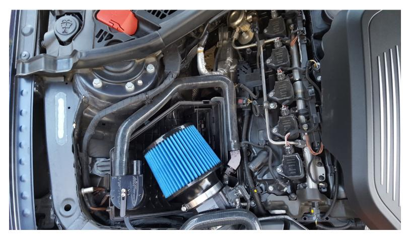
Place the other hose on the "in" nipple of the oil catch can. Then place the other end on the valve cover nipple shown in the photo below. This is a very low pressure system so hose clamps are not needed.
