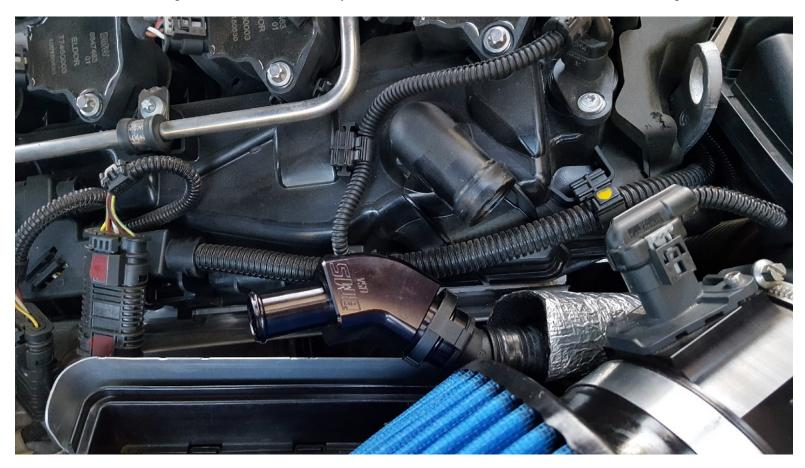
Now place the hose shown below on the "out" of the oil catch can (it's labeled next to the nipples) to the PCV hose with the BMS adapter.
