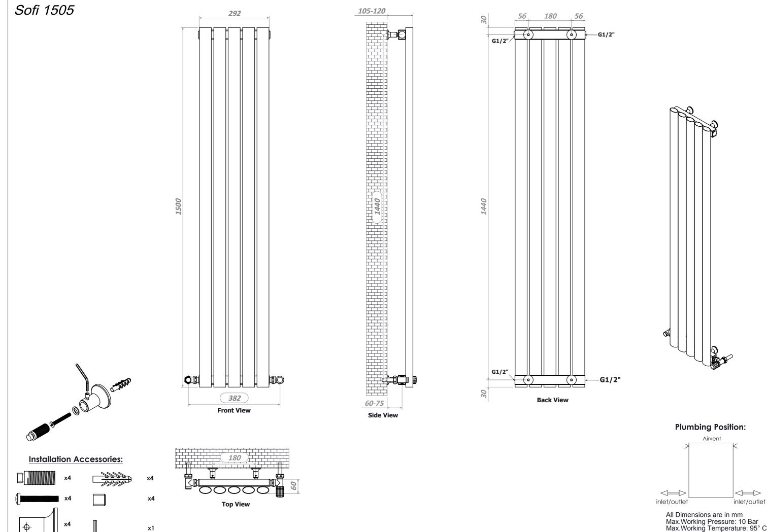
All Dimensions are in mm Max.Working Pressure: 10 Bar Max.Working Temperature: 95° C Inlet / Outlet : 1/2" BSP Fuel : E/H/D
