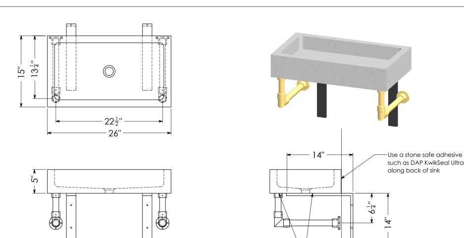
Use a stone safe adhesive such as DAP KwikSeal Ultra along brace top, and where brass attaches to sink
