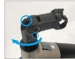
1. Adjust the top and side screws so that the riser rotates to face straight ahead
