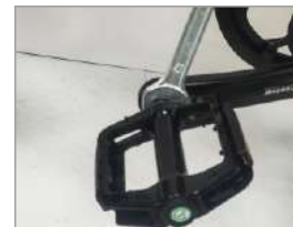
8. Take out the pedal with the letters "R" and "L", align it with the crank hole and lock it with a wrench
