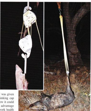
(Left) Starting from scratch with JackStrap rigged up in the dark, the simplicity of JackStrap ensured a perfect result first time. (Inset) JackStrap close up at maximum lift height. Note this system has a fairly short head height (the distance from top anchor to the load).
