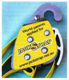
The top block of the JackStrap. The aluminium lever just below the hook is the automatic, inertiaoperated locking piece. Note how small the hook is, necessitating the use of a small chain or wire to attach it to a beam.
