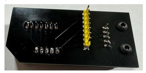
Slide the sensor mount into the top case making sure the male and female haeader align correctly. Secure the sensor mount in the top case using three strands of filament, trimming each one flush with the case.
