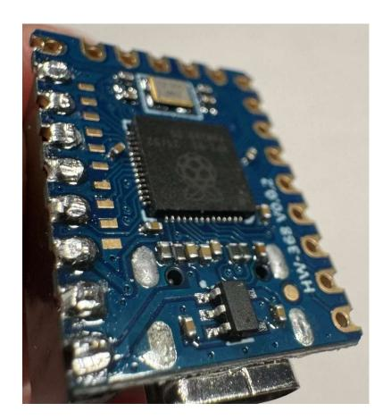
Install the RP2040-Zero into the bottom case and secure with a strand of filament. You can leave a little extra filament hanging out on this one if you like.
