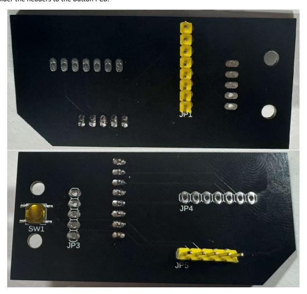
Place the Button PCB over onto the sensor mount insuring that the header pins align with the holes and solder in place.
