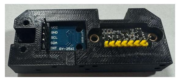
Using four strands of filament, secure each board in place. Trim the filament flush with the side of the sensor mount.
