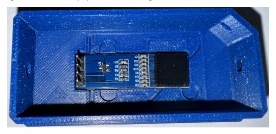
Make sure the display is fully in the pocket by checking that there are no gaps on the front of the unit.
