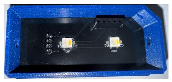
Trim the leads as flush as you can. Take care not to damage the LED or the resistor next to it.
