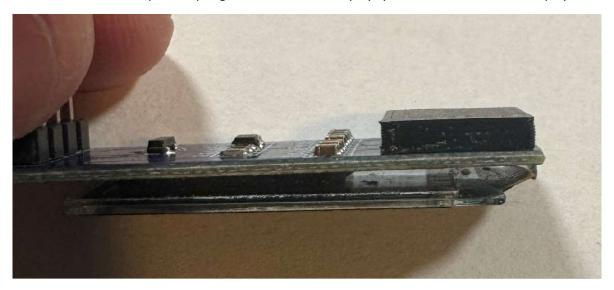
Gently insert the display into the slot. This may take some time to get the display to align with the pocket as it's a tight fit to insure the display does not shift during normal use.
