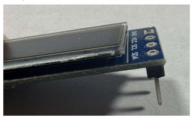
Use some double sided tape or super glue to adhere the display spacer to the back of the display.
