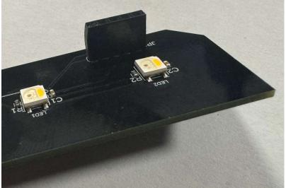
Set the LED PCB down on top of the display, making sure the leads slide through the the holes.
