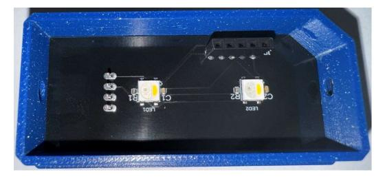
Solder the display leads while the LED PCB is in place.
