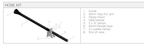
Other hose kits and filters are available. All of the above units are fitted with our standard filter combinations. For specific applications please call us for details. Replacement filters should always be ordered using the part number on the filters inside your extractor to ensure the correct filter is ordered. Datasheet correct at time of print.
