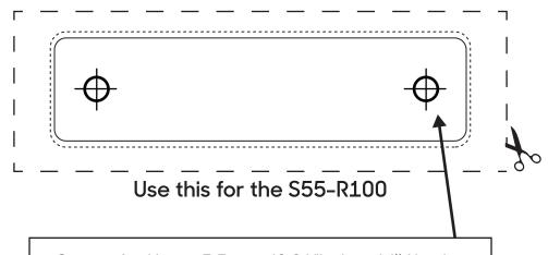
Option 1 - Use a 5.5mm (0.21") size drill if using the enclosed 5mm bolt/washer/nut.
