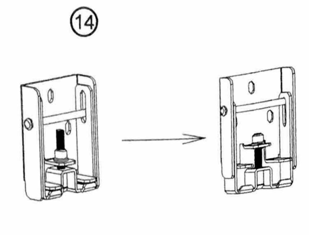
3.Screw the lower brackets to the wall, the distance between the upper bracket and the lower bracket is "A" minus 15mm or 3/5 inch, For example, if your frame "A" measurement is 1270mm or 50 inches. Then the top of your top bracket to the bottom of your bottom bracket (with the bottom bracket screws tightened) would be 1255mm or 49 2/5 inches. the distance between the two lower brackets is "B" minus around 1000mm or 40 inches (for reference)
