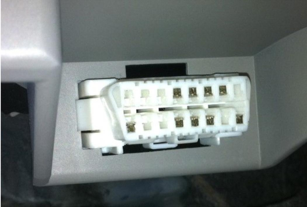
Connect the OBDII cable with green end into this port, and the connector into the Handheld. CAREFULLY.
