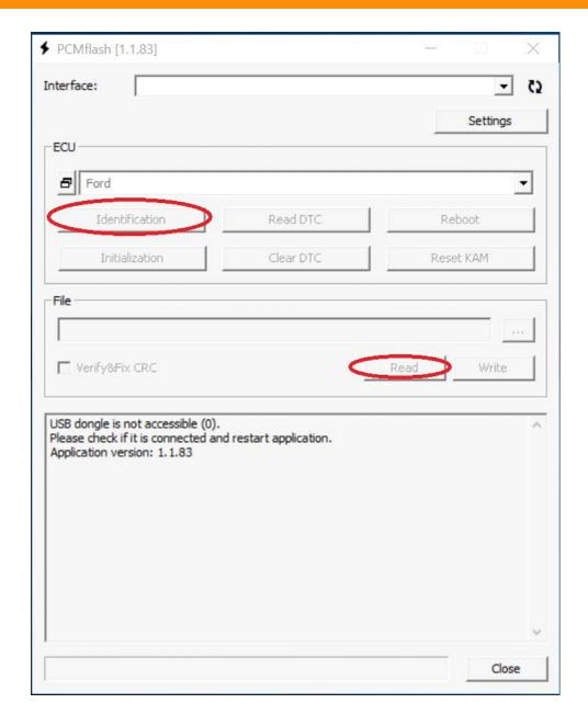
The Writing process is nearly identical. To ensure you are securely connected to your ECU press the IDENTIFICATION button and allow it to read your ecu calibration information.
