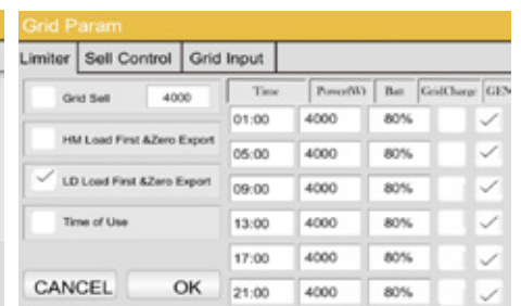
6. Set HM Load & zero export, set grid charge and discharge time
