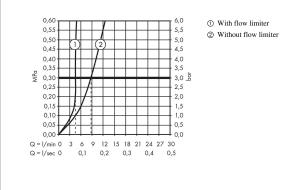
$\begin{array}{c} 6.0 \\ 5.5 \\ 5.0 \\ 4.5 \\ 4.5 \end{array}$  With flow limiter
