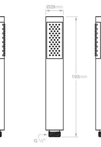
Dimensions given are in mm. LIQUIDRed® reserves the right to alter and /or remove designs from time to time without prior notice. This drawing is to be used for reference purposes only. E &O.E.
