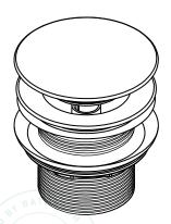
Base Material: Brass Mechanisim: Press to Pop-up Plug Type: External Dome Cover Pipe Thread Connection: G 11/2" (40mm) Use: Bath Waste with thick wall base
