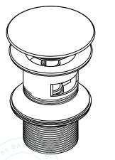
Base Material: Brass Mechanisim: Press to Pop-up Plug Type: External Dome Cover Pipe Thread Connection: G 11/4" (32mm) Use: Basin Waste, with overflow
