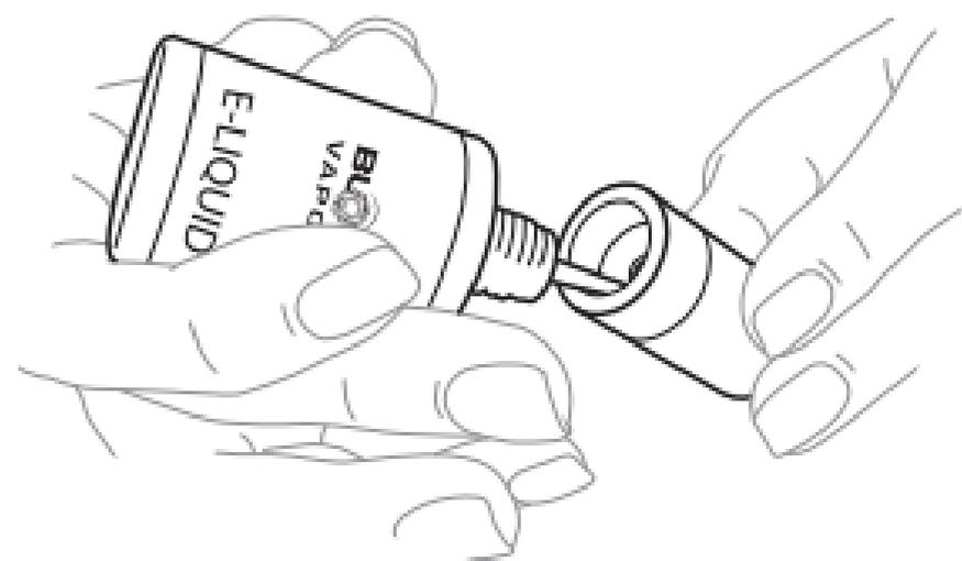
2. Fill Blow Vapor's E-Liquid into the Tank about 3/4 to the top.
