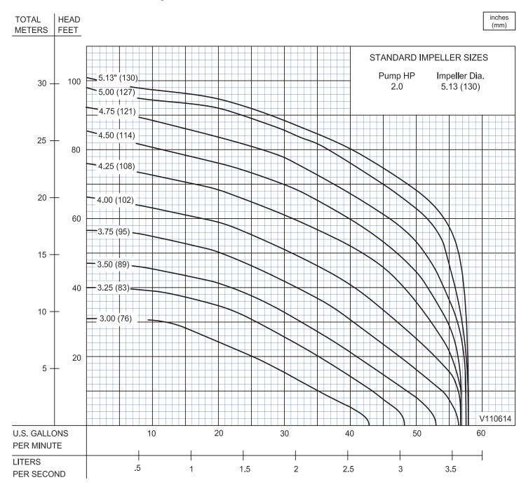
Testing is performed with water, specific gravity 1.0 @ 68º F @ (20°C), other fluids may vary performance
