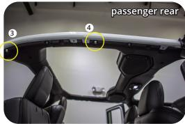
Use the leverage strap to pull the shock cord in-between the Power top and the roll cage. This will be a snug fit.
