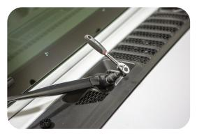
Use the ratchet in the Jeep® toolkit provided to remove the (4) T40 windshield bolts and carefully lower the windshield onto the hood pads.
